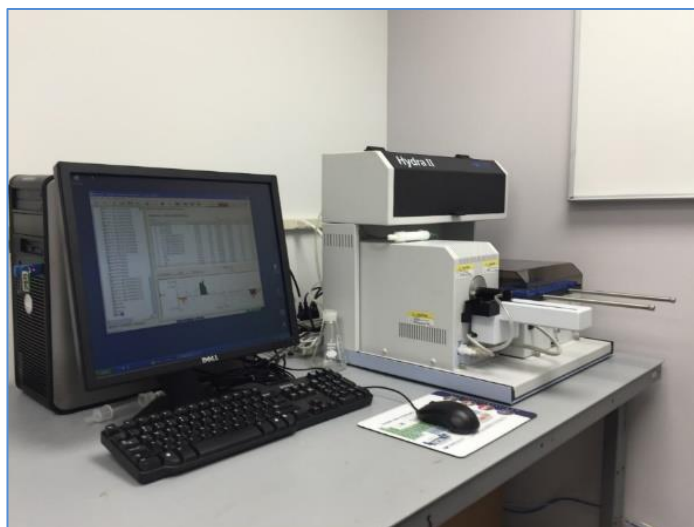
Figure 9 Hydra II c Combustion Atomic Absorption (CAA) Mercury Analyzer in a Typical Laboratory Setting
