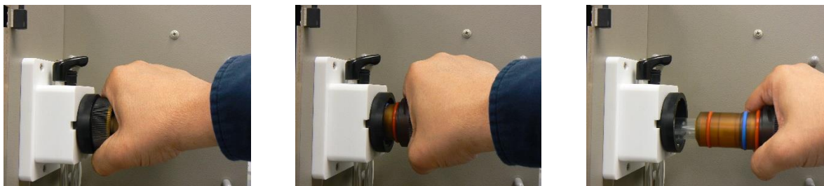
Figure 2 Axial Twist Lock Sample Introduction System
