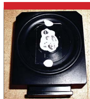
Figure 1: Lead fragments mounted in a laser cell.
