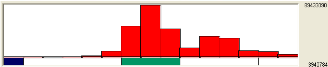
Figure 2. Graphical Representation of the Be 234.861 nm Subarray for the 10 ppm Calibration Std
