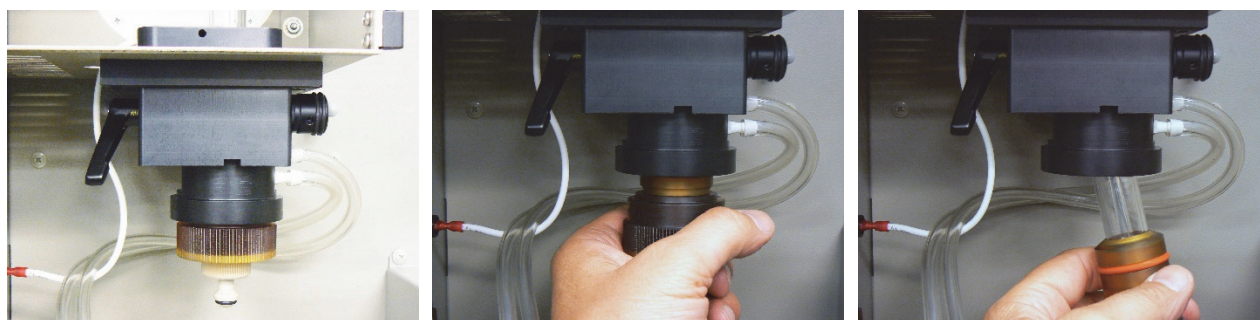
Figure 3 Radial Twist-n-Lock Sample Introduction System
