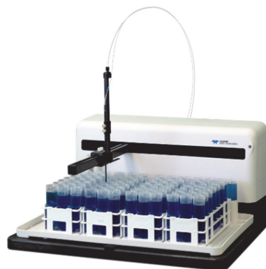
Figure 2 Teledyne CETAC ASX-560 Autosampler
